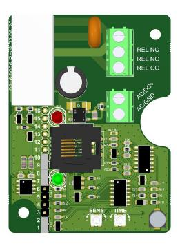
The RJ12-plug connector is provided for direct connection to the sensor switching module (SENSOR plug socket). A suitable switchpoint can be adjusted with the "SENS" potentiometer. The switch-off delay can be set using the "TIME" potentiometer.
